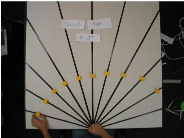
Figure 2 Measuring the on-table reach envelope
