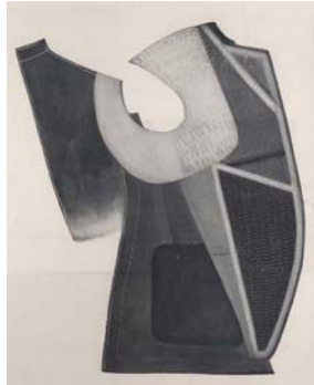
Figure 3: The Interior of a Suit Jacket, Showing Layers of Stitched Padding and Interfacing
